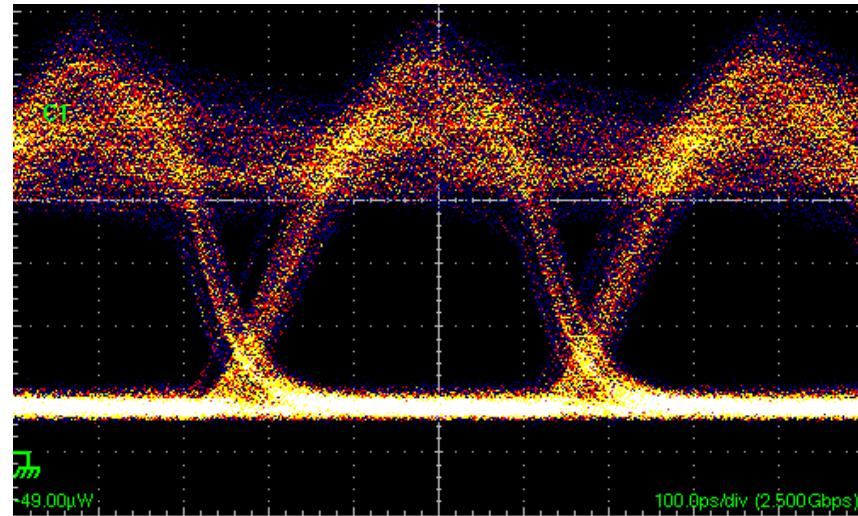
2.5 Gb/s NRZ 2<sup>7</sup>-1 PRBS electrical signal applied,  $\pm 4$  V swing, 4 V DC bias
