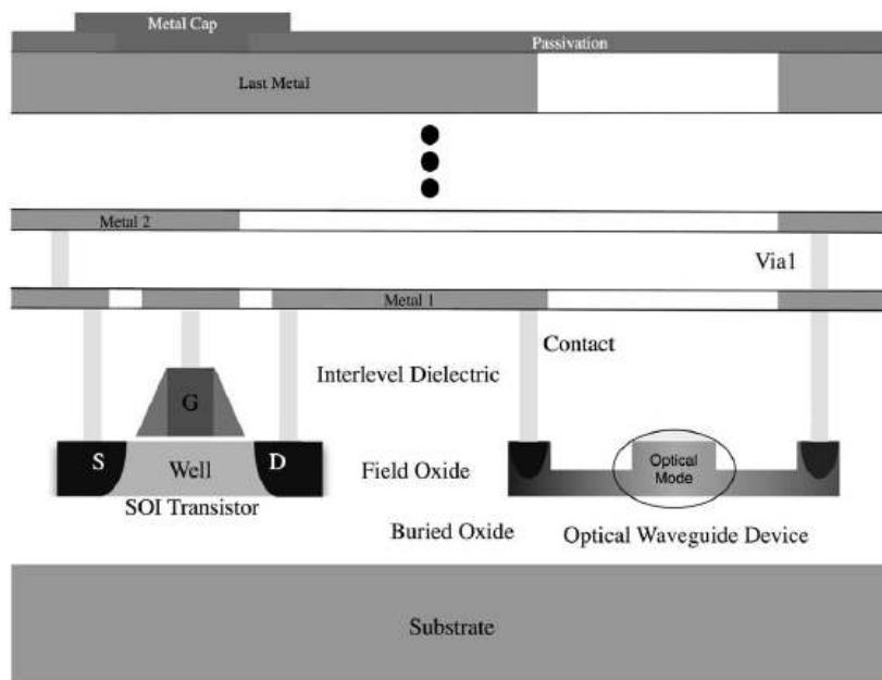
Figure 1. Schematic cross-section of SOI CMOS Photonics process
