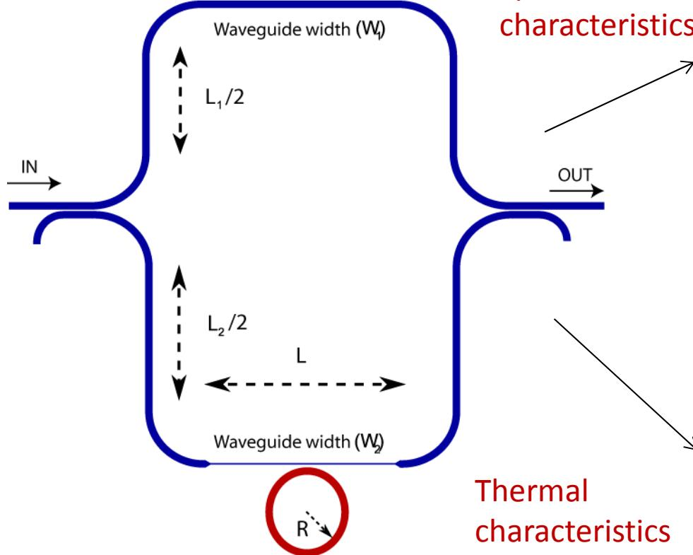
Ring resonator overcoupled to a balanced MZI
