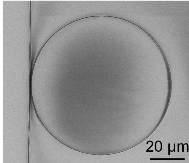
700 nm waveguide width, 40  $\mu\text{m}$  radius
