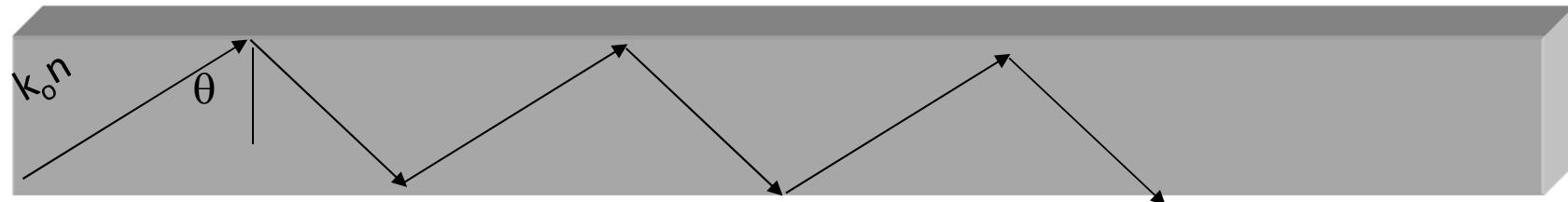
$$2k_o nh \cos \theta + \phi_{\text{down}} + \phi_{\text{up}} = q2\pi \quad q=1,2,3\dots$$
