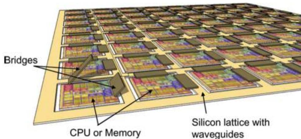
Fig. 1. Macrochip is a logically contiguous piece of densely interconnected silicon that integrates CPUs, memory, and a systemwide optical interconnect.
