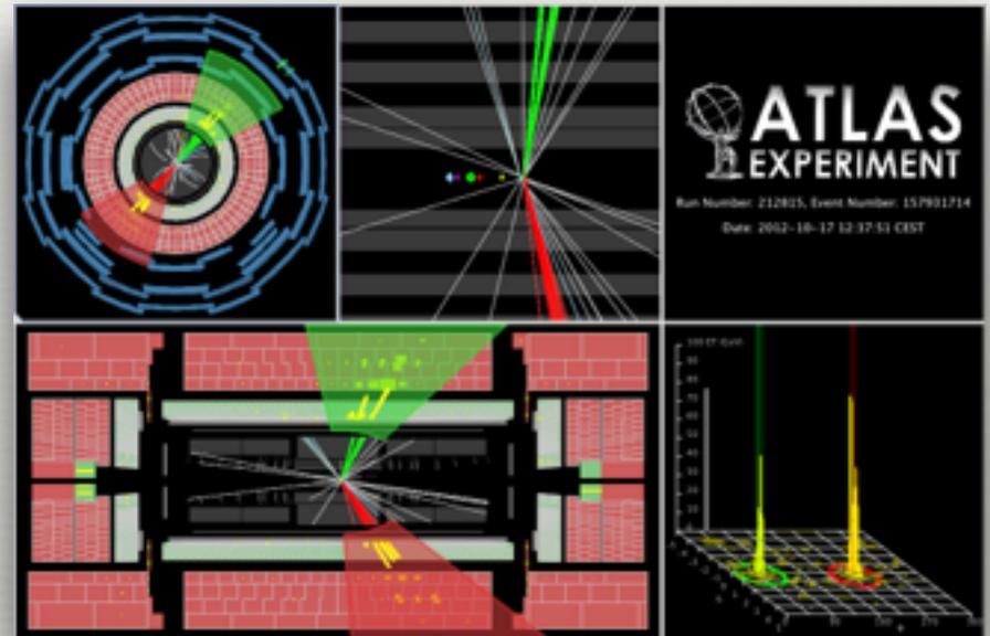
Atlas event selected by the WW, WZ and ZZ cuts, with dijet invariant mass  $m_{jj}=2.0\text{TeV}$ . Leading jet has  $P_T=1.1\text{ TeV}$  and  $m_j=93.7\text{ GeV}$  while subleading jet has  $p_T=0.9\text{TeV}$  and  $m_j=92.8\text{GeV}$
