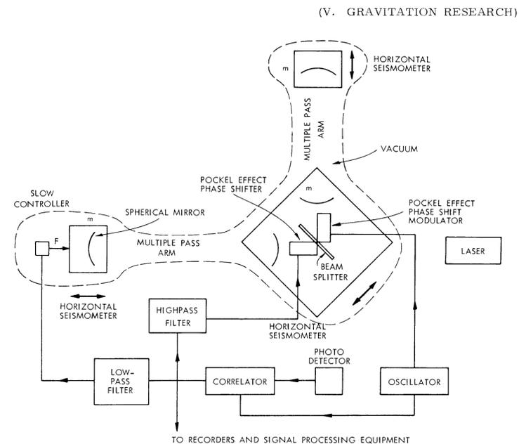
Fig. V-20. Proposed antenna.
