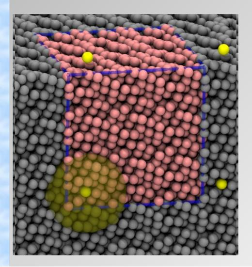
Cubic box of particles with a Lennard-Jones type pairwise additive interaction potential
