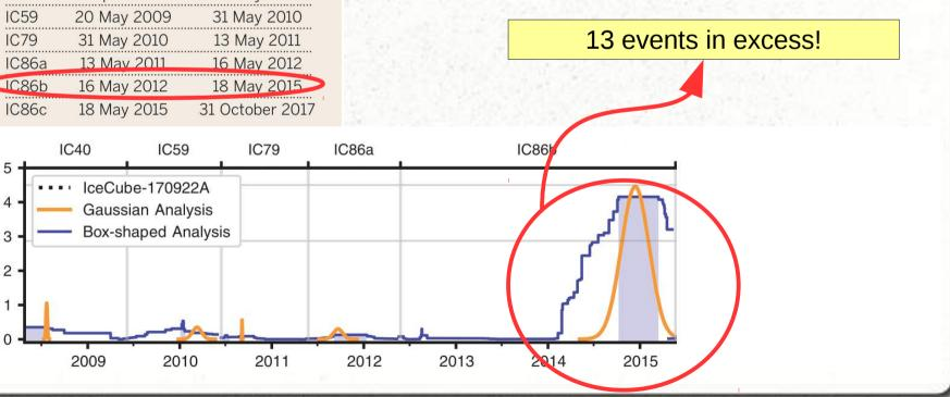
Six data-taking periods make up the full 9.5-year data sample. Sample numbers correspond to the number of detector strings that were operational. During the first three periods, the detector was still under construction. The last three periods correspond to different data-taking conditions and/or event selections with the full 86-string detector.
