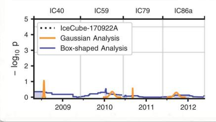
Six data-taking periods make up the full 9.5-year data sample. Sample numbers correspond to the number of detector strings that were operational. During the first three periods, the detector was still under construction. The last three periods correspond to different data-taking conditions and/or event selections with the full 86-string detector.
