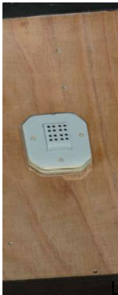
Recessed positioner; fibers on this side, MPPC on other side
