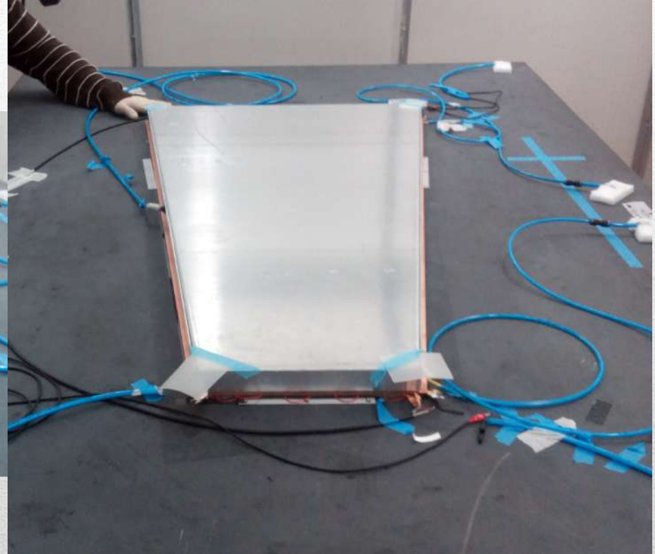
Chamber with aluminum honeycomb strong-back
