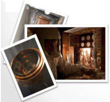
DAMA/LIBRA: 250 kg crystals of ultra-pure sodium iodide (Thallium doped)
