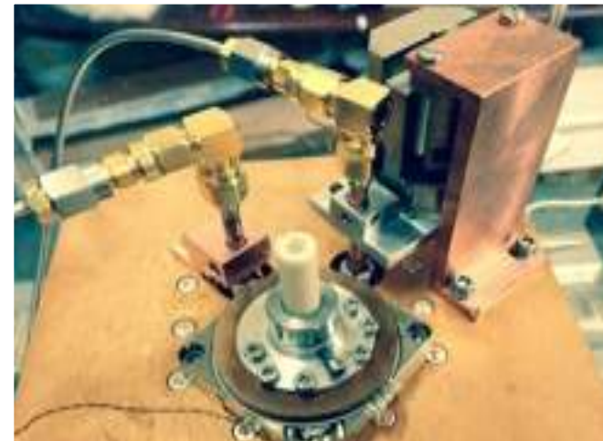
4-6 GHz Test Cavity with piezo actuators at U. Washington
