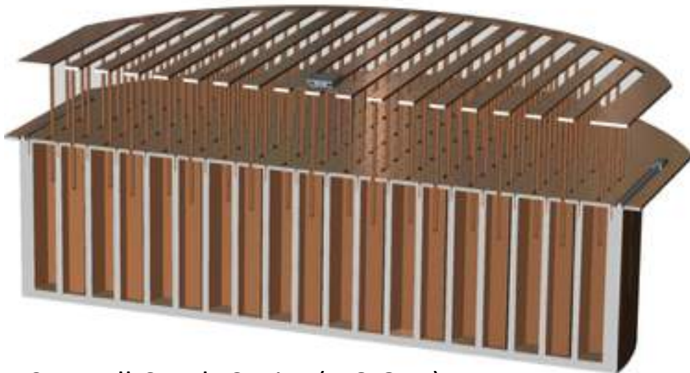
241 cell Comb Cavity (4-8 GHz)
