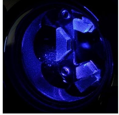
Figure 4.10: Picture of a strontium MOT operated at 461 nm. The atomic cloud, which consists of about 10^6 atoms at 10 mK temperature is visible as a diffuse spot located inside a three-mirror ring cavity (courtesy: Camila Beli and Michelle Moreno).
