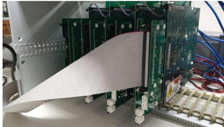
Low Threshold Acquisition (LTA) readout electronics
