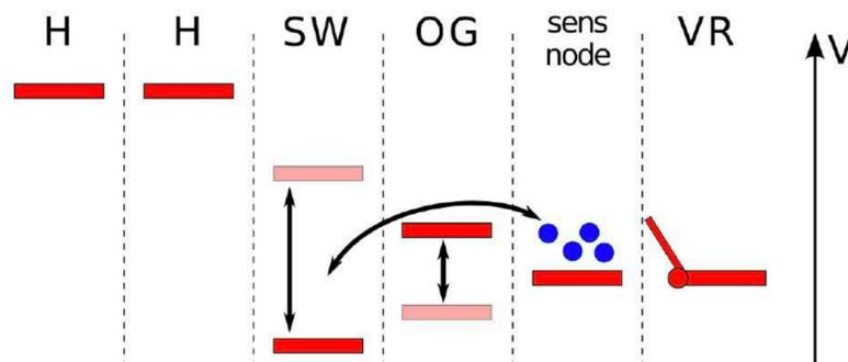
multiple readings of the charge of the same pixel
