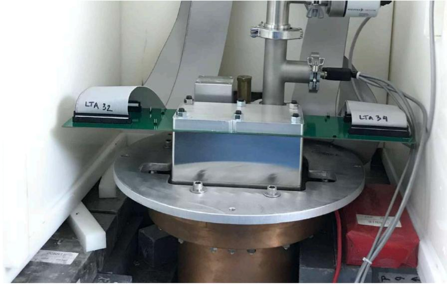
New vacuum interface board installed
