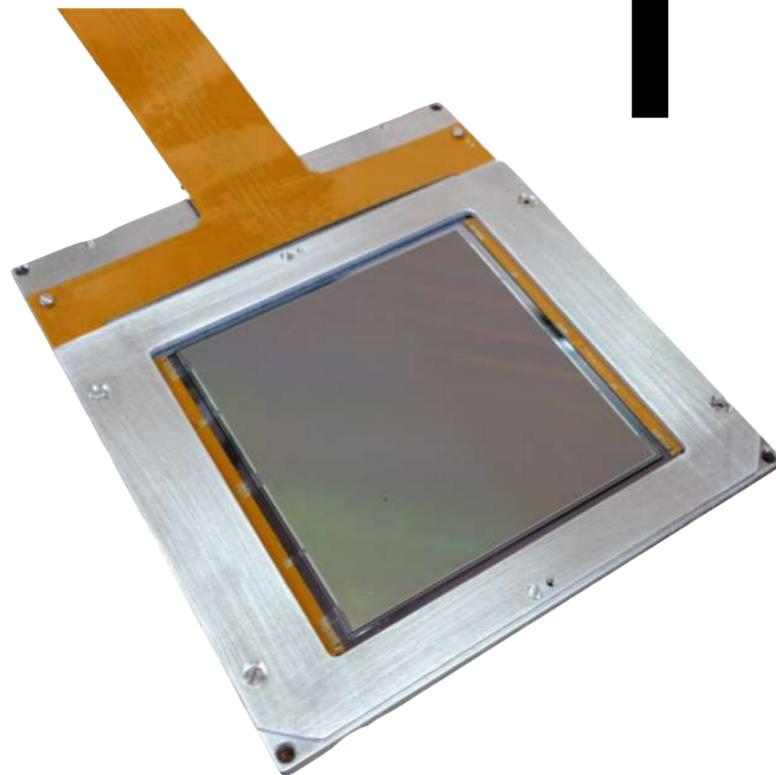
16 Mpix CCDs with  $15\ \mu\text{m} \times 15\ \mu\text{m}$  per pixel
