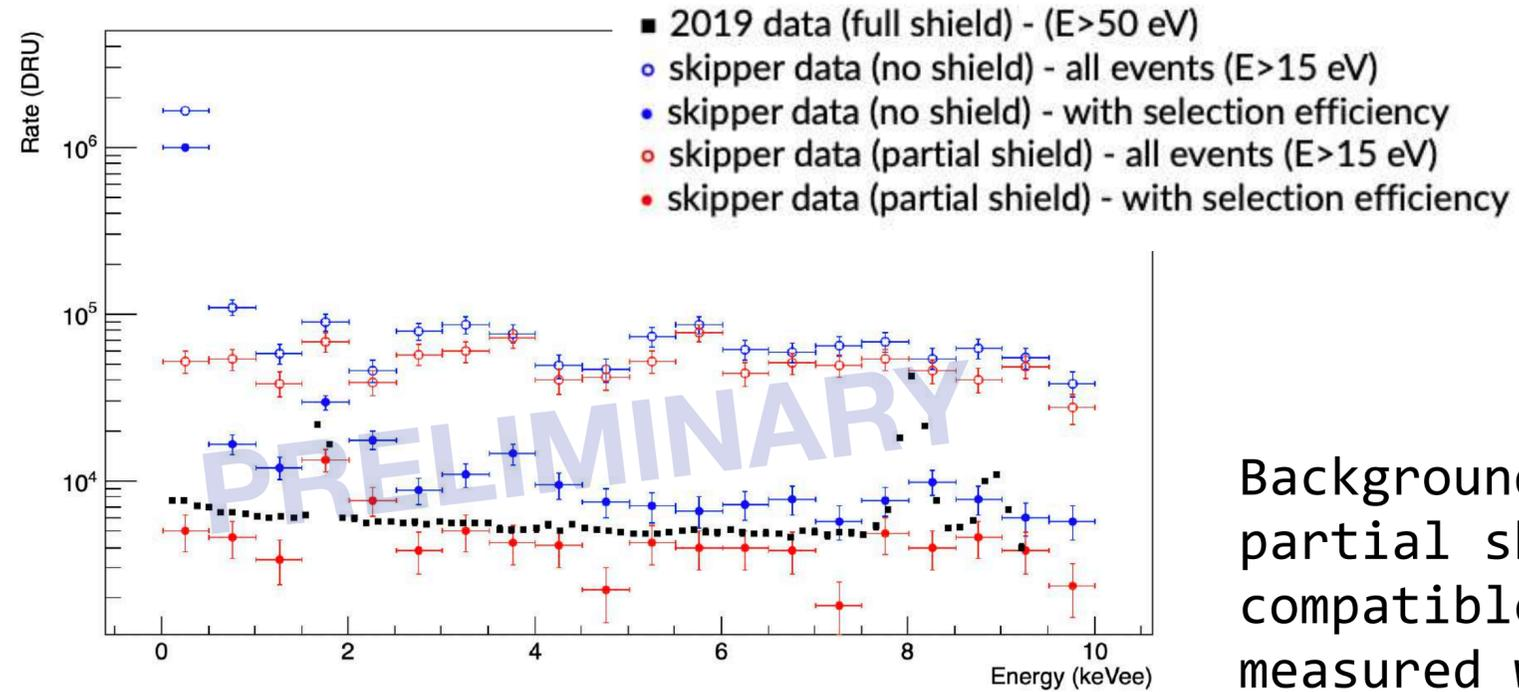
Background measured with partial shielding is now compatible with the background measured with 2019 data
