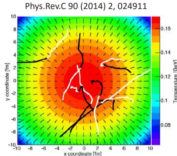
Illustration of few  $c\bar{c}$  pair trajectories in the expanding medium after  $10 \text{ fm}/c$
