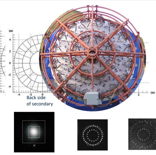
Actuators system for mirror alignment
