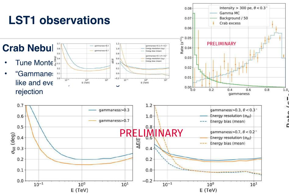
Angular and Energy resolution of LST1 using tuned MC to Crab Data and source independent analysis.
