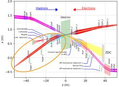
IP magnets, Lumi & low-Q<sup>2</sup> detectors
