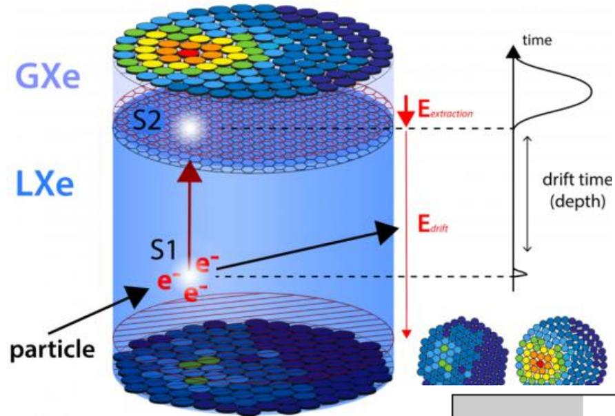
Liquid xenon time projection chambers searching for WIMP dark matter at Gran Sasso with 3.9-4.1 t (XENONnT) and Jinping with 2.5 t (PandaX-4T)
