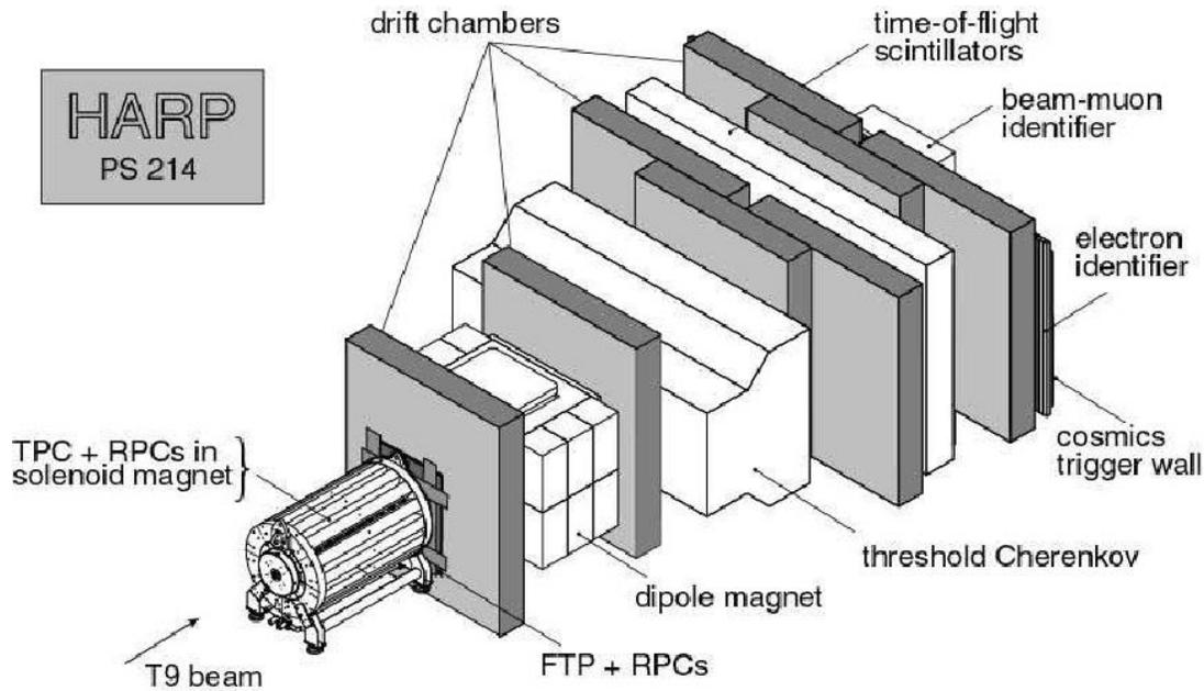
HARP experiment at CERN studied meson production from p-nucleus collisions on multiple nuclei providing final-state kinematics
