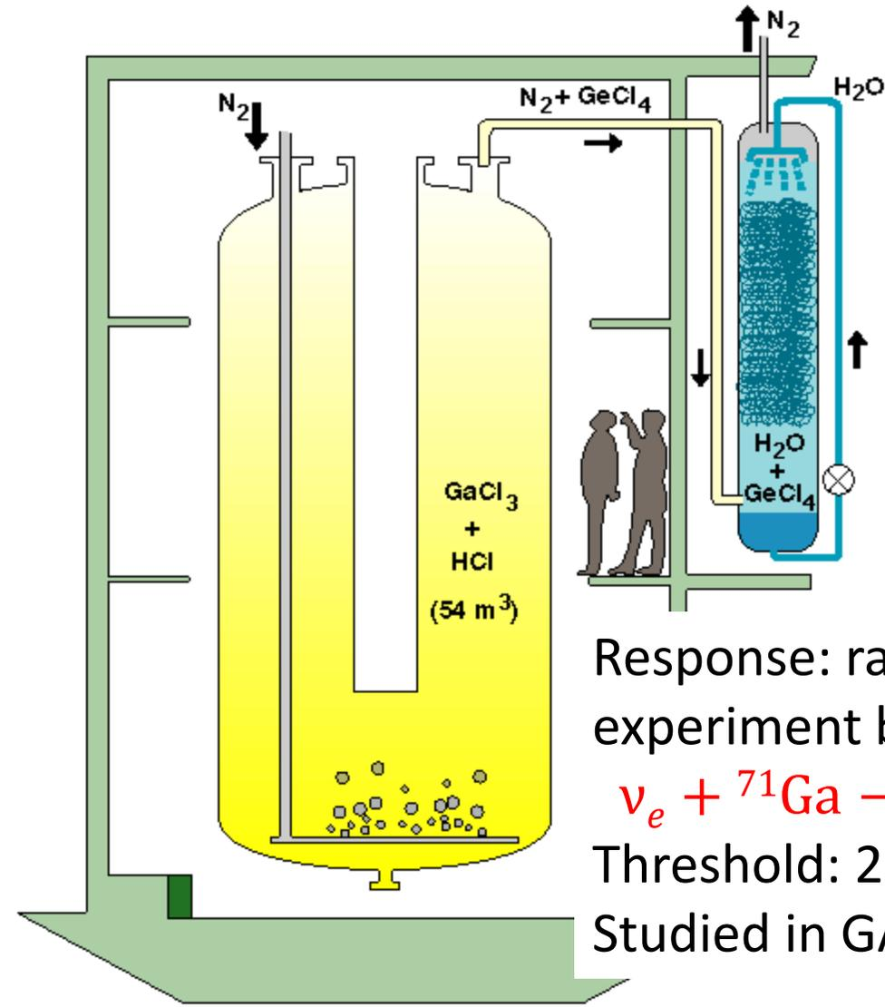
Response: radiochemical experiment based on Ga
