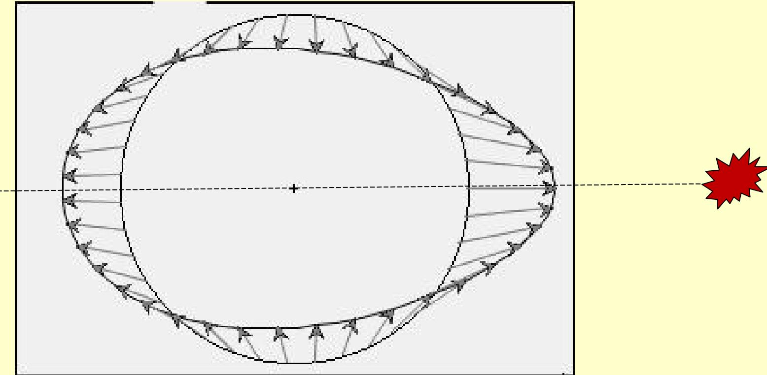
If the distance to the external body is much larger than the dimensions of the body, the deformation tends to be symmetrical.
