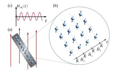
$$\hat{H}_{0}(t) = \sum_{i} \left( J_{i} \hat{\sigma}_{i}^{z} \hat{\sigma}_{i+1}^{z} + \sum_{\alpha = x, z} h_{i}^{\alpha} \hat{\sigma}_{i}^{\alpha} \right) + \sum_{n=1}^{\infty} \delta(t - nT_{S}) \phi \hat{S}^{x},$$
