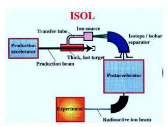
Online separation: thick target + ion source + separator + post-accelerator
