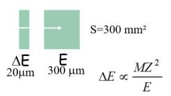
Second solenoid helps cleaning the secondary beam: degrader changes the Bp of the particles with different Z (q)
