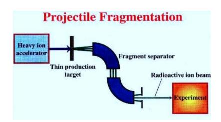
In-flight production: thin target + separator
